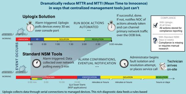
policy engine to determine if a parameter is in or out of specification. Uplogix can then either automatically resolve the incident based on pre-approved automated operations, or communicate information back to centralized IT staff for resolution management tools. All of this happens in less time than most standard management tools take to find the problem, and often before users even knew there was an issue.
